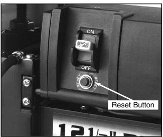
Figure 5. Location of switch and reset button.
